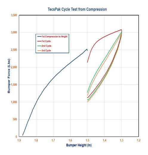
For this example, the bumper was compressed to the installed height (1.50 inches) and allowed to dwell for five minutes. The bumper was then cycled between heights 1.30 and 1.50 inches for three cycles. As can be seen, with this method, the bumper continues to take a lower load at the installed height of 1.50 inches.
