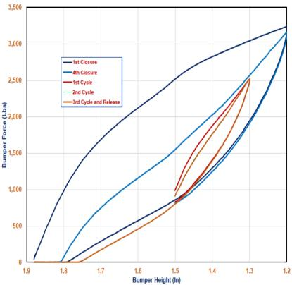
TecsPak Cycle Test from Release Curve
